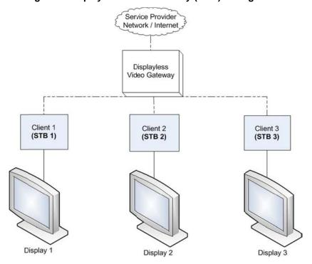
Figure 2: Displayless Video Gateway (DVG) Configuration
