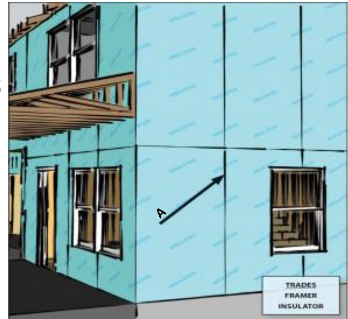
Example: Continuous rigid foam insulation installed
