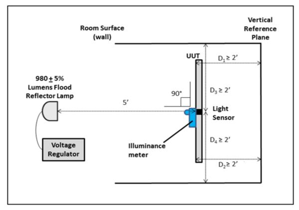
Figure 2: Test Setup - Top View
