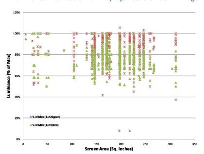
Figure 1: Luminance Distribution for Displays Less than 30" in Diagonal Size
