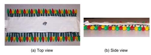
Figure 1. A mounted decorative light string prepared for testing.
